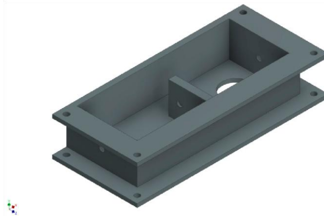
Figure 14. Creation of the holes that support the axle of valves B and C.
