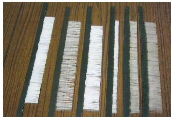
Fig. 2 Trailing Edge Serrations (Oerlemans et al., 2009)
