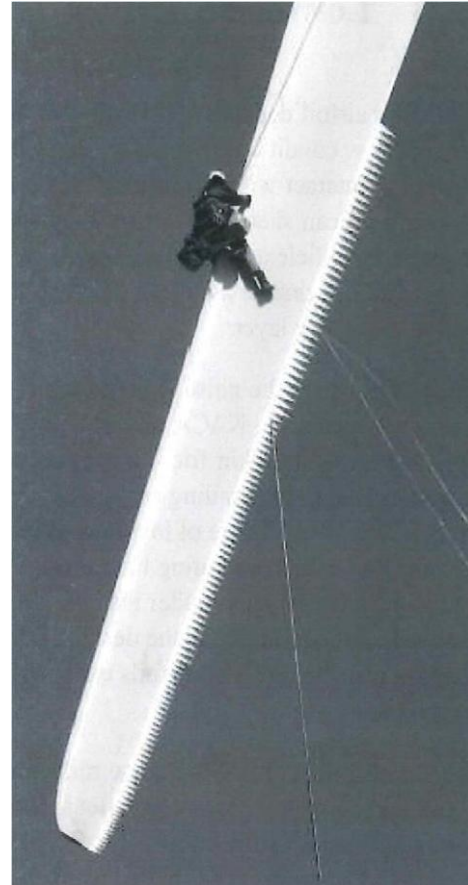
Fig. 2 Trailing Edge Serrations (Oerlemans et al., 2009)
