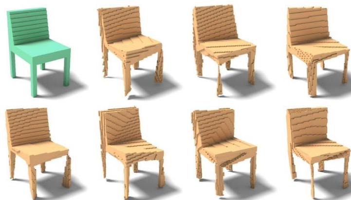
FIGURE 9. A series of random vertex displacement distribution limited to the 5% of the voxel space width.
