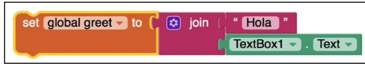
Figure 5. An App Inventor code snippet with LOC=2 and LLOC=1.
