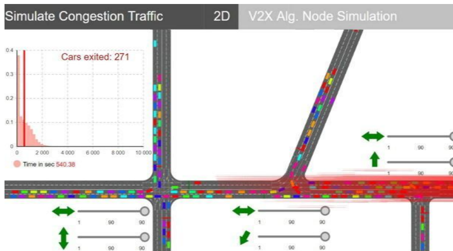
Figure 7. Congestion scenario 2—vehicle flow generated on 300/min, 90 s of red traffic light.
