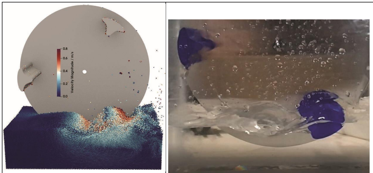
Fig. 6: Results of numerical simulations using smoothed particle hydrodynamics (l.) showing a washing machine paddle diving into water compared to test bench investigations (r.)
