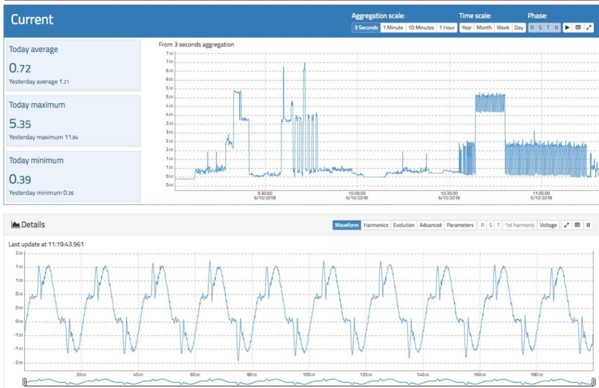
Figure 11. View of root mean square (RMS) and waveform current in oZm.
