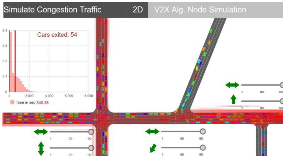
Figure 11. Congestion scenario 4—vehicle flow generated on 700/min, 90 s of red traffic light.
