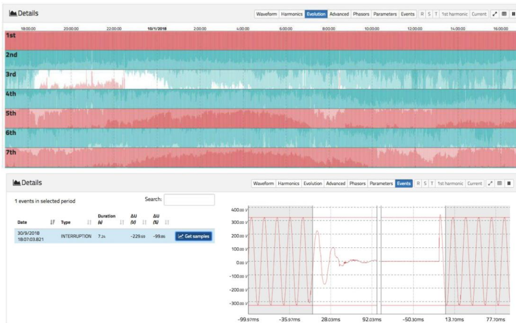
Figure 10. Advanced views of voltage tab (2). (Top): harmonic evolution. Darker red colours indicate higher values than darker blue. (Bottom): events view with pre- and post-event waveforms.
