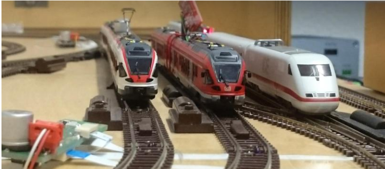
Fig.6. The physical demonstrator component. Shown are the modified model trains with the Bluetooth-LE (red PCB) back-channel to notify balise detection for odometry. The IRDA balises are seen in the foreground tracks between the white ribbon-cables connected to the IR-PCB.
