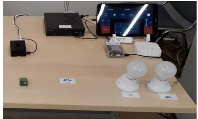
Figure 4 IIoT Testbed infrastructure, showing the Controller node, IoT gateways, smart sensor and actuators (smart lights)
