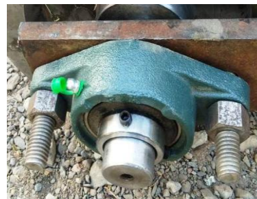
Figure 6.2 Actual placed Bearing
