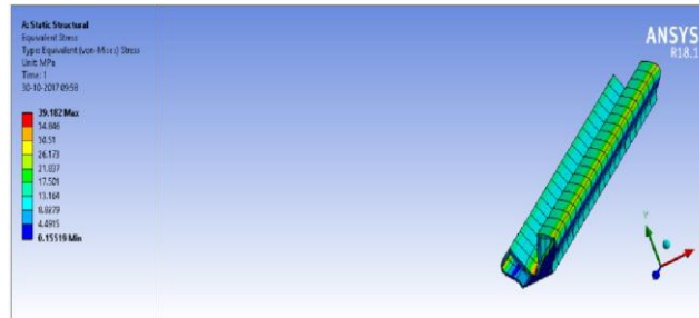
Figure 25 Frame Materials analyses on Ansys
